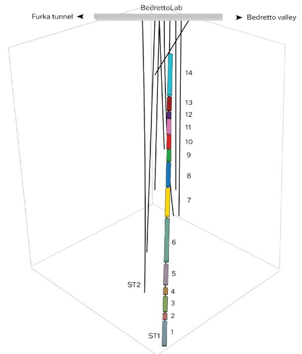
Top: Boreholes in the Geothermal testbed and intervals in the 399-meter long ST1 stimulation borehole.
