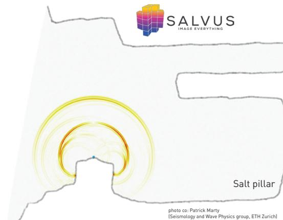
*Synthetic wavefield using the SALVUS model for a point source on the salt pillar surface. Models will be used to absolutely calibrate the acoustic emission sensors – the same sensors that will be used for the FEAR experiments in the Earthquake Physics testbed*
