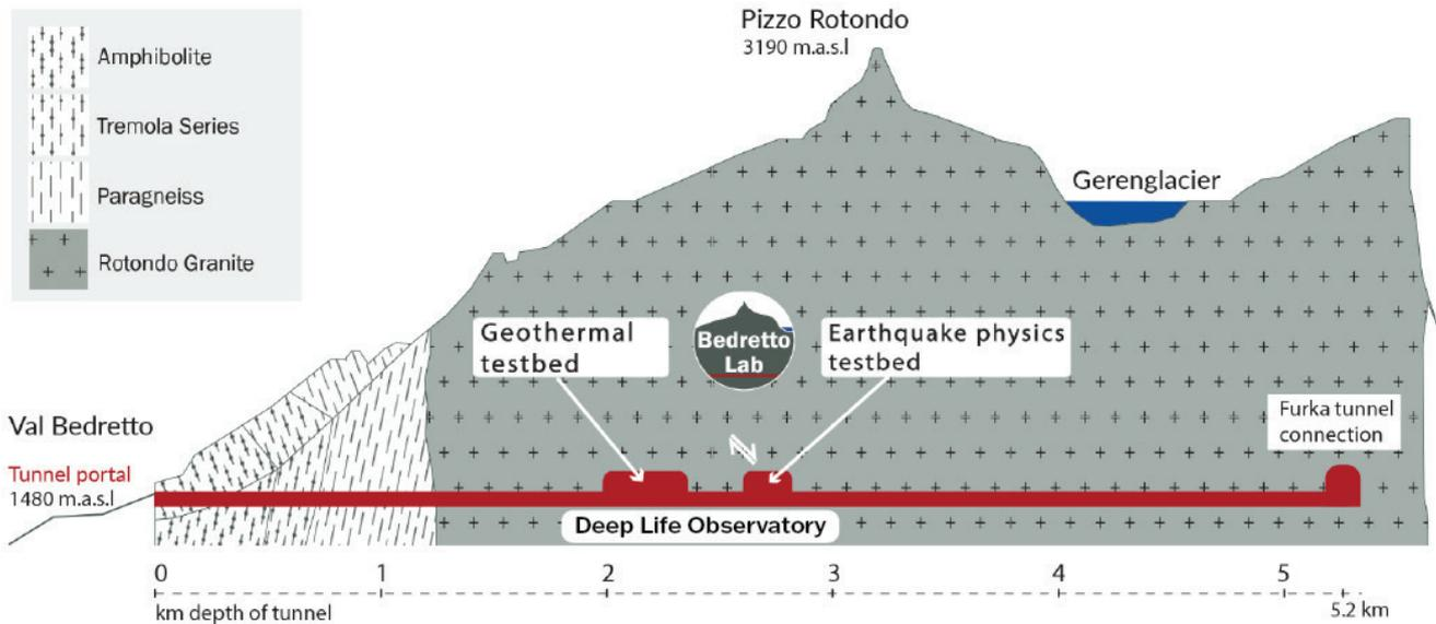
**Geothermal testbed**, focusing on the development of large-scale deep reservoirs for water circulation, storage and extraction of geothermal energy.
